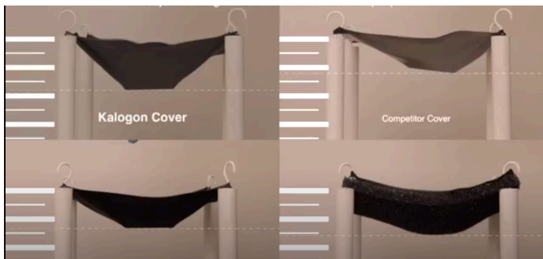
Figure 13: Example of a Qualitative Cushion Fabric Comparison Test to Evaluate Stretch.
